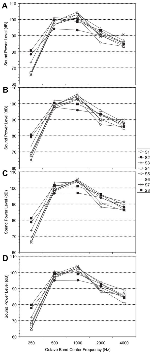
**FIGURE 4.** Octave band sound power levels of the singers measured in the reverberation room for the four singing modes A to D.
