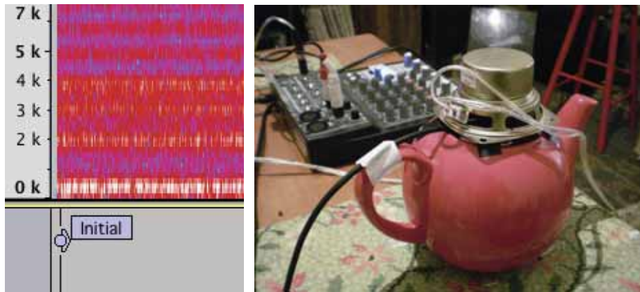
Figure 4.13 (left) Spectral analysis by the author of the white noise signal in the Red teapot during the initial recording, the lighter bands indicate a stronger amplitude response – hence the resonant frequencies of the teapot. (right) The Red teapot being recorded in July 2009.
