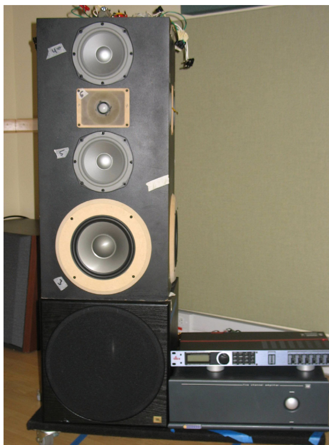
Figure 1 A photograph of the adjustable loudspeaker with its electronics, showing the L2 configuration. Note that the top midrange driver is not active for this configuration.
